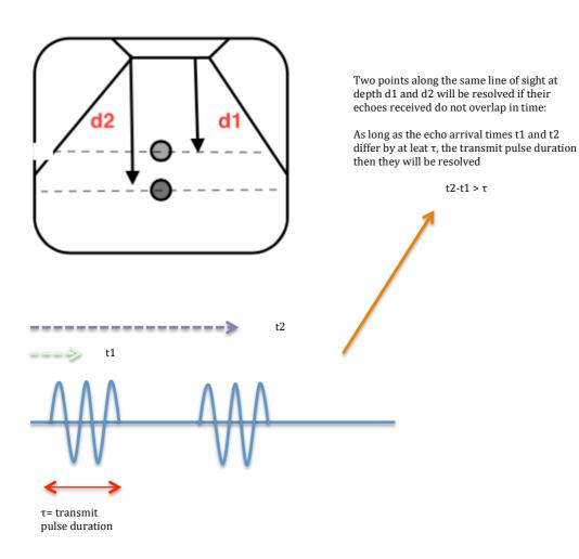
Utilising the pulse echo principle: t = 2d/c
