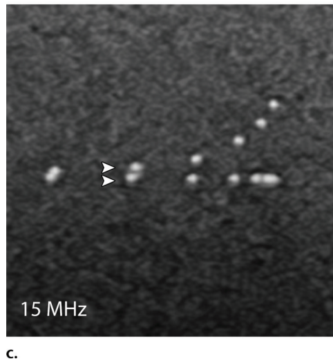
Figure 4. Axial resolution. (a) Diagram shows the relationship of axial resolution to the SPL, which is inversely related to frequency. Arrows = beam path over time. Top: A single beam approaches two targets (red bars). Middle: If these targets are separated by a distance greater than one-half the SPL, they will be resolved. Bottom: If the separation is less than one-half the SPL, the returning echoes will overlap and they will not be resolved. (b, c) US images of echogenic foci (arrowheads) in phantoms demonstrate an improvement in axial resolution when the frequency increased from 9 MHz (b) to 15 MHz (c).
